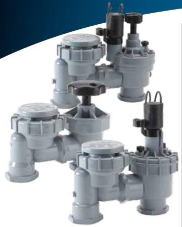
The Irritrol® anti-siphon 2700 Series valves offer optimum performance, reliability and ease-of-use for a wide variety of residential applications. Featuring anti-siphon capability, this family of plastic valves also features flow control for precise flow adjustment, manual shutoff and a built-in atmospheric vacuum breaker to eliminate back siphonage. Available in electric and manual models, these valves also feature a flow range from .25 to 30 GPM and a pressure range from 10 to 150 psi.
